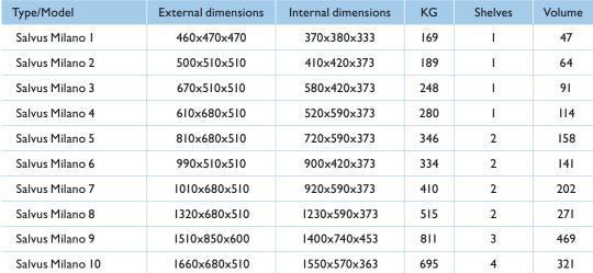
External depth does not include 48 mm for door handle and hinges
